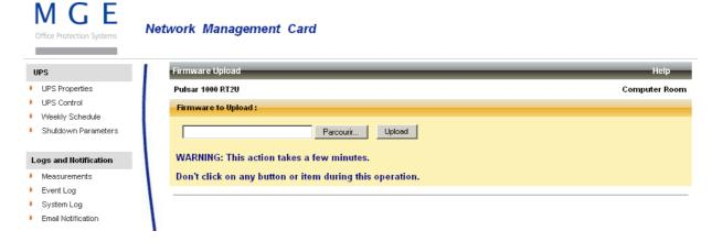
To upload a new version of the card's firmware, select the file to be loaded using the "Browse..." button and click Upload.
